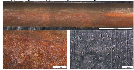
Despite of very low water content clear corrosion effects
