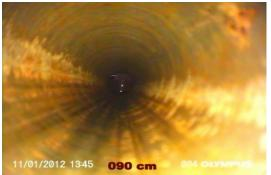
1000 h, 50 °C, 150 bar, 2 m/s CO<sub>2</sub>, 25 ppm H<sub>2</sub>O, 25 ppm SO<sub>2</sub>, 0.8 % O<sub>2</sub>
