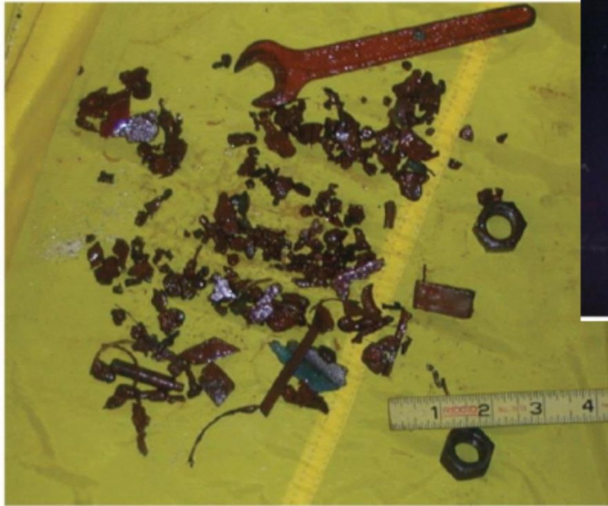
Debris found in a feedwater heater where a fretting fuel failure occurred
