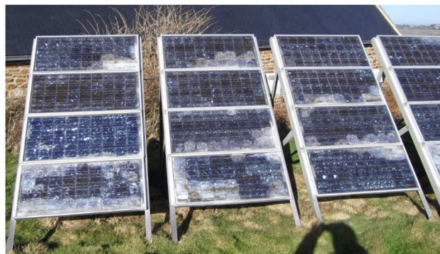
FIGURE 1 Salt deposit on solar panels in coastal climate (photo: Daniel Lincot). [Color figure can be viewed at wileyonlinelibrary.com ]
